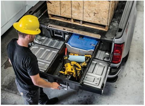
The Vehicle Storage System from DECKED<sup>®1</sup> provides a durable and organized storage solution for pickups or cargo vans. The system features smooth-rolling, secure drawers with customizable storage options that still allow use of the cargo area.
